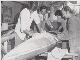
FIBERGLASS —Industrial education students at Northern Arizona University are busily making a fiberglass kayak which costs $40 plus a lot of work. From left, Tom Post, Flagstaff, IE instructor; Jerrie Jenkins, Payson; and Don Saffey, Cottonwood. A canoe costs $80 to build and can be in the water two weeks after a student starts on the project. Once a mold is made, almost anything can be made from fiberglass.
